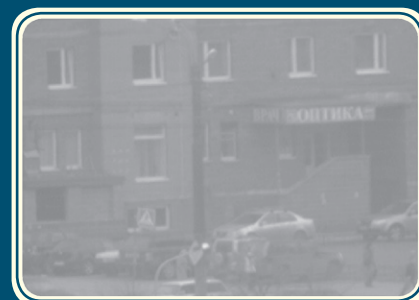
Illustration of the fog surveillance with the density of the fog 15db/km with the WAT-902H (top) and VSC-751 (bottom). The distance to the object in the central zone is about 1,5 km.
